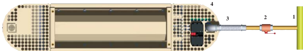
Fig. 18 Diagram of the connection of the SUNRAD emitter to the gas network
